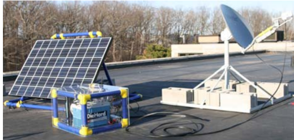
Figure 1. IMAGINE prototype ground station being tested in Ann Arbor, MI. This prototype was used to develop and solicit funds for the field units shown in Figure 2.
